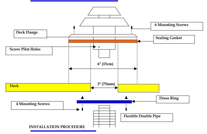
**Step - 1** Cut a 3" hole through the deck, ceiling or wall.
