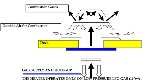
If there is a propane fuel system installed a separate supply line must be supplied for the heater. This line must be equipped with a low-pressure regulator (Dickinson Part No. 19-151)
