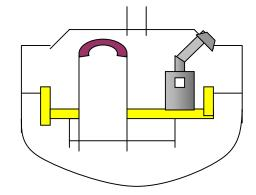
**LOCATE** the heater where it will maximize the radiant heating capability. The NEWPORT PROPANE HEATER is equipped with a manually operated blower fan that will blow hot air from the top of the heater down onto the floor. This increases heating efficiency and provides good circulation of hot air.
