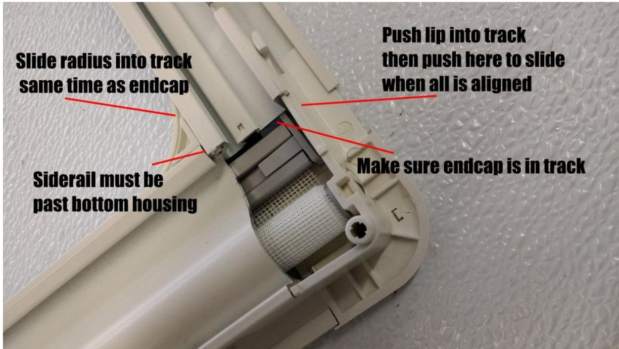
To finish, pull both shade and screen to make sure it glides properly through track. Put on liner if needed.
