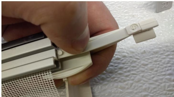
Slide handle until the nib click into hole in xbar
