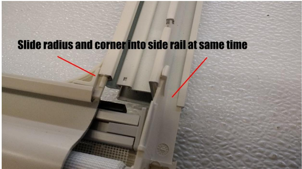
The corner will not slide if siderail is not past bottom housing. Make sure the endcap of X-bar is in track. You can the press below the notch to allow corner to slide on. Keep finger away from notch to not pinch your finger. Do this to both ends making sure the notch click into siderail.
