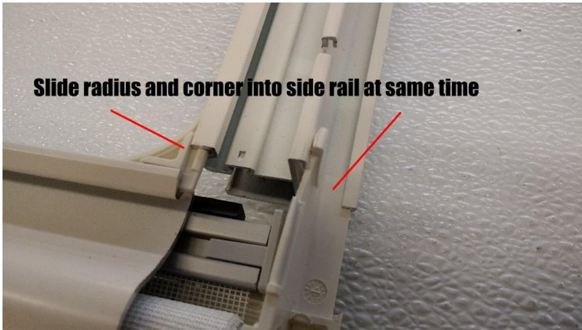
The corner will not slide if siderail is not past bottom housing. Make sure the endcap of X-bar is in track. You can press below the notch to allow corner to slide on. Keep finger away from notch to not pinch your finger. Do this to both ends making sure the notch click into siderail.
