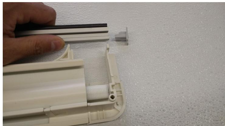
Use a soft tip hammer to not scratch. Hit handle where it meets crossbar to knock it over notches
