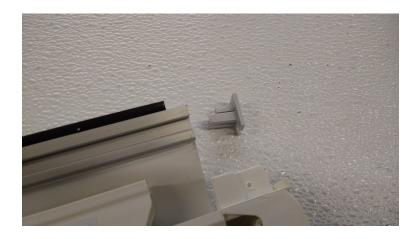
Use a soft tip hammer to not scratch. Hit handle where it meets crossbar to knock it over notches
