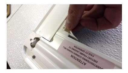
Snap the radius back into siderail and end cassette slit . Put on liner if needed.
