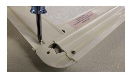
Put siderails back into corners and tighten screws
