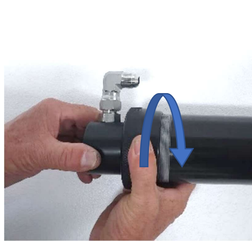
2-Thread the Ring on until the End Cap Seal contacts the Tube
