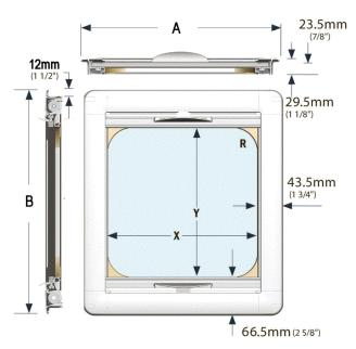
When selecting a SKYSCREEN ROLLER RECESSED it is important to establish the type and manufacturer of hatch, aperture dimensions (X&Y), overall dimensions (A&B), mounting location and interior design.
